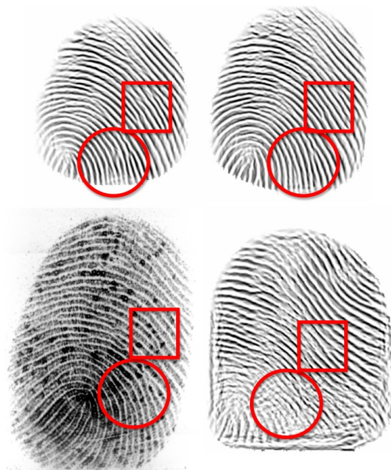
Figure 7. Clean print on a normal fingerprint sensor (lower left) images, and 3 examples from an image with significant spatial image processing. Compare the structures in the circled and squared regions. We really don't know what causes the very distorted images like the lower right, where even the overall flow is wrong.
