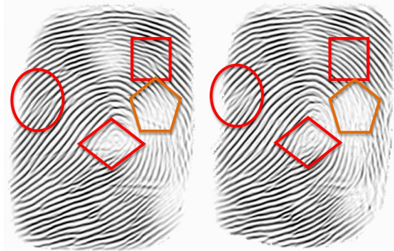
Figure 6. Images captured from the same finger using a sensor with advanced spatial image processing. The image output by the sensor looks great, but has hidden dangers. The minutiae in red colored region represent different minutiae information for the same finger.
